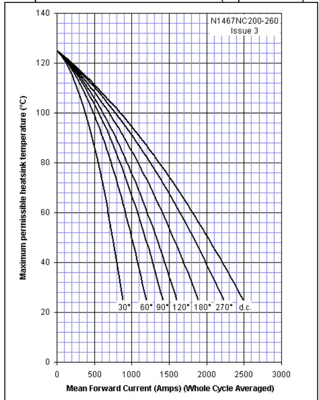
Figure 9 – On-state current vs. Power dissipation – Single Side Cooled (Sine wave)
